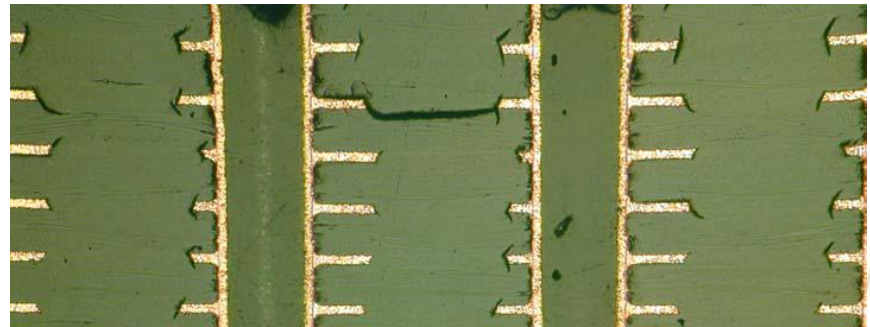
Example of Delamination (I)
