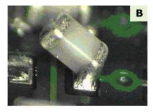
The higher temperature can also cause delamination of multilayer PCBs and damage components.
